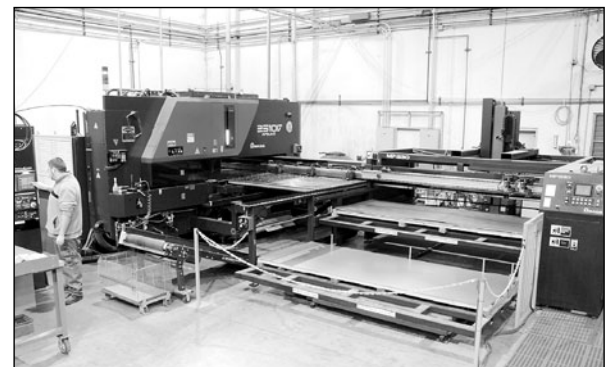
A variety of flat parts is produced quickly, in mass quantities, by this Apelio combination punch and laser. Note the automatic sheet feed and parts conveyer.
