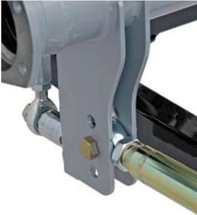
This factory photo shows how the other end of the trailing arm attaches to the axle bracket using spherical joints, which offer zero deflection. The length of the trailing arm is adjustable at this juncture, and the adjustment is locked into place with the large jamb nut.
