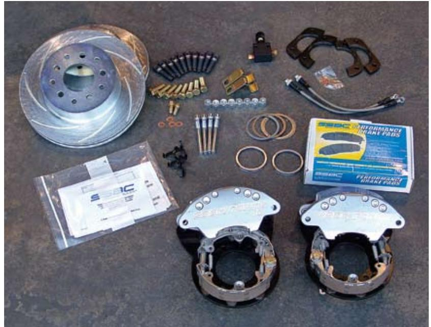
During the course of the conversion, we'll also install these rear disc brakes from Stainless Steel Brakes Corp. Included along with the calipers are slotted rotors, parking-brake assemblies, and braided steel brake lines.
