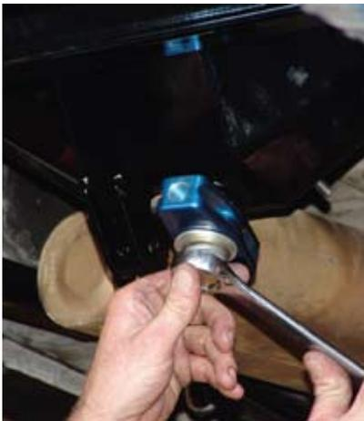
The pivot arm for the Watt's linkage is mounted to a threaded boss welded onto the bottom of the FAB9 housing or to your supplied housing.
