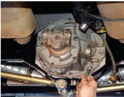
As you can see, the arms of the Watt's linkage have been installed going from the pivot arm out to the bracket on the end of the axlehousing. Here we see the Currie 9+ third member going into place.
