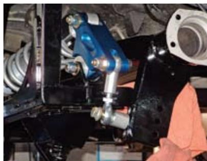
This photo shows the shock-absorber connection on the outside end. For this project, a new Chris Alston FAB9 housing will be used, but the axlehousing of your choice can be easily equipped with the required mounting bracketry using the included brackets, instructions, and your MIG welder.
