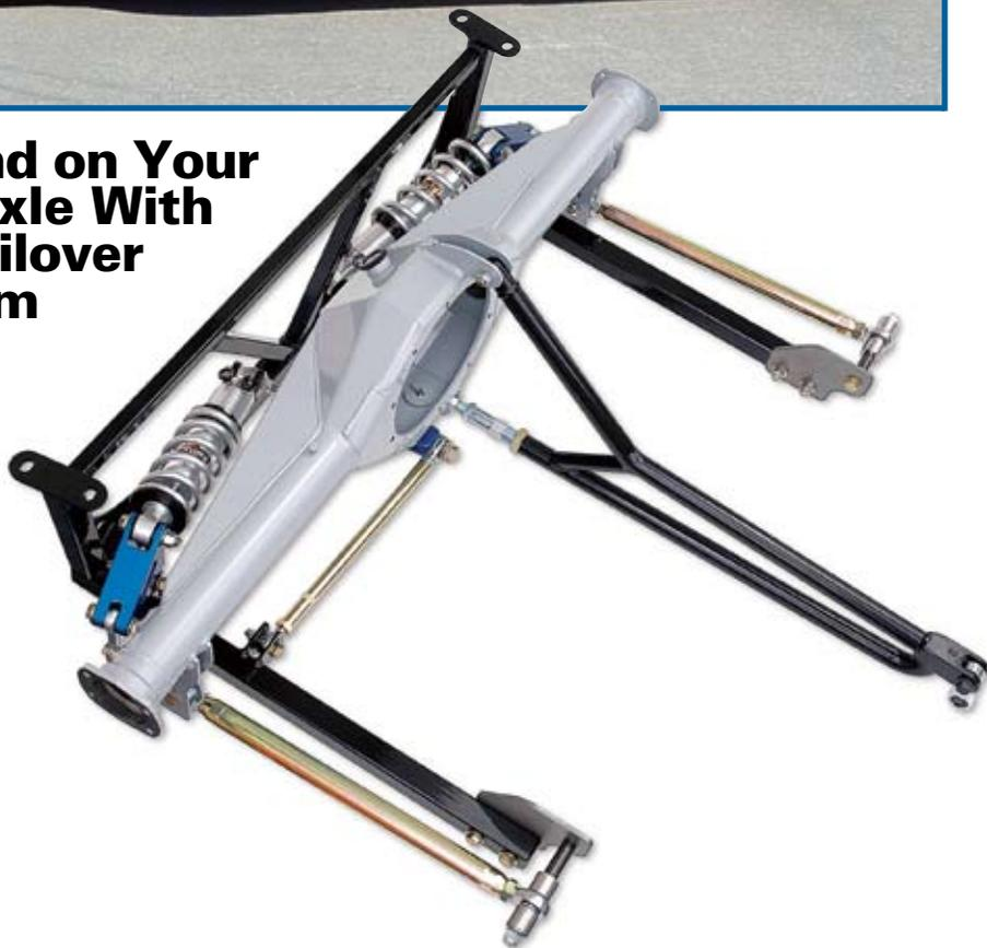
When performance-oriented people install larger wheels and tires out back, it becomes clear that the leaf springs are a limiting factor when it comes to selecting a tire and offset for any kind of high-performance application, be it road racing, drag racing, or just spirited driving. The original leaf-spring suspension also allows serious axle windup, and it does a poor job of locating the axle precisely in relation to the chassis during turns.
