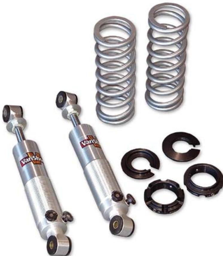
Here's a close-up of the coilover shocks. Besides allowing the ride height to be dialed in exactly via the threaded adjustment collars, they're also externally adjustable for both bump and rebound in a range covered by 16 increments.
