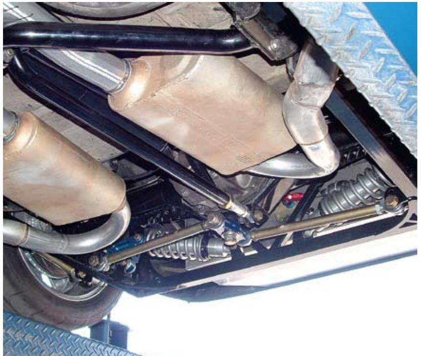
The Total Control Products suspension is in place. All that remains is to set some final adjustments, making sure the rearend is centered and squared. Then it's time to go road racing. Mustang Depot opted for an Eleanor-type side-exhaust kit for its project. Other exhaust solutions include simple turndowns at the mufflers or short tailpipes that dump into the rear wheelwells.
