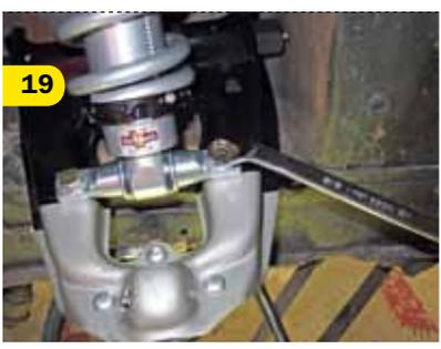
With our new upper control arm installed and bolted back into the shock tower, the final step is to mount the coilover to the upper control arm. If you're reusing a good control arm the stock spring perch will need to be removed, of course, but our new upper arm was already sans spring perch.
