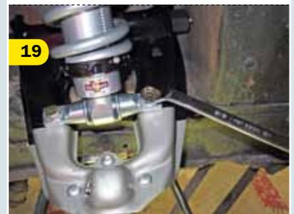
With our new upper control arm installed and bolted back into the shock tower, the final step is to mount the coilover to the upper control arm. If you're reusing a good control arm the stock spring perch will need to be removed, of course, but our new upper arm was already sans spring perch.
