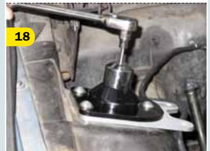
TCP offers these polished coilover mount covers if you're looking to add a little shine to your installation. They install easily by removing the coilover's grease fitting and securing the mount cover with the included Allen screw into the grease fitting hole.
