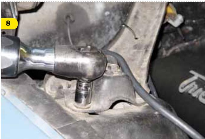
With our shocks assembled, we can now move forward with disassembly of our stock components—mainly the shock and coil spring. Remove the shock mounting cap retaining nuts (the mounting caps will not be reused). We're installing TCP's Tower Export Brace kit as well, so we're removing the stock braces at this time, too.
