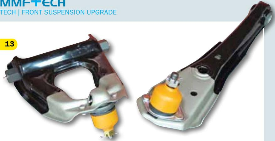
A quick call to Mustangs Unlimited solved our ball joint problem. Mustangs Unlimited suggested Scott Drake's new show-quality control arms. While far from a show car, these new control arms are built with OE level steel in the right thickness with high-quality riveted ball joints—just what the High School Hauler needs!
