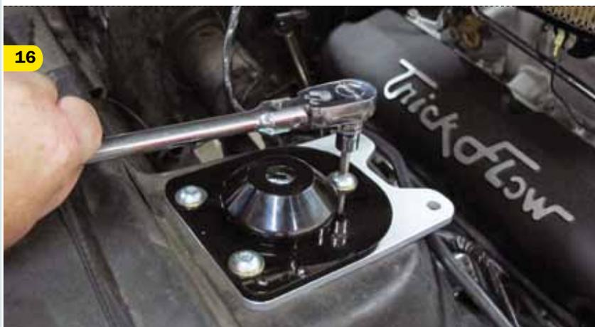
The coilover upper mount sandwiches the shock tower. The upper plate is placed over the shock opening while the backing ring is installed from inside the shock tower. If you're installing TCP's Tower Export Brace kit as well, you'll have to decide whether you want the mounting plate above or below the coilover plate. Mounting it below, as we have, lowers the front suspension approximately another 1/2-inch.
