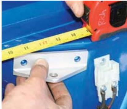
**3** Monte Carlo bar installation calls for close attention to detail because it must be spot on. Because inner fender aprons can vary in how they were stamped, especially reproductions, bracket positioning can get tricky.
