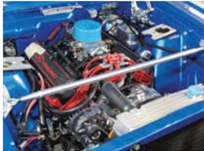
**12** Here's the final installation of the Monte Carlo bar.
