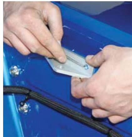
**7** Perform a test fit before drilling holes for the left side Monte Carlo bar bracket. Make sure your bar will be dead straight end to end.
