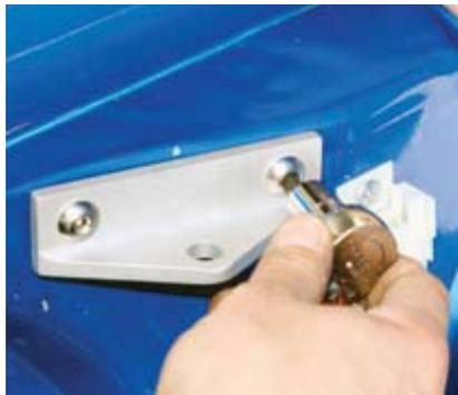
**4** On the right-hand side, you want the Monte Carlo bar bracket parallel with the top of the battery apron with the front bolt hole around 10 1/2 inches from the trailing edge of the radiator support. Bracket should be approximately 1/8 to 3/16 inch below the top of the apron.
