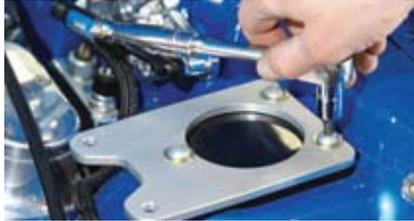
**1** Because Project Reclaim has already been fitted with a TCP coilover front suspension, we're going to have to remove the shocks to install our TCP export brace. Billet brackets sit on top of TCP shock brackets. Allen screws retain the export brace brackets along with locknuts underneath.
