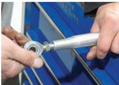
**11** After screwing in the Heim joints, the Monte Carlo bar can be installed. Adjust Heim joints for stiffness, but don't overdo it. Lock down the stop nuts.
