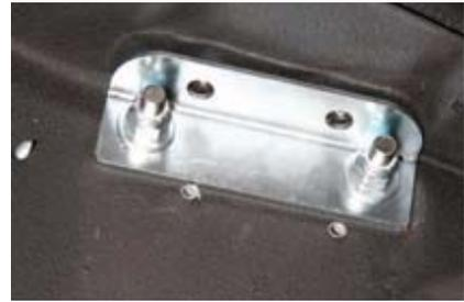
**5** Underneath, this support bracket should be installed as shown. Once it is secure, the top bolt holes are drilled, first as 1/8-inch pilot holes, then the full 3/8-inch.
