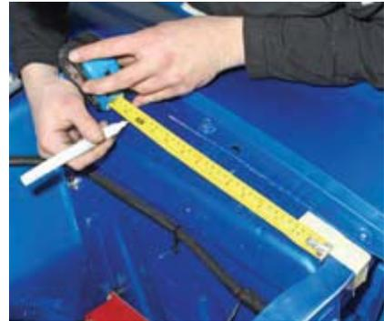
**6** Follow the same procedure on the left-hand side, with the Monte Carlo bar bracket located with the forward bolt hole at approximately 10 1/2 inches from the trailing edge of the radiator support.
