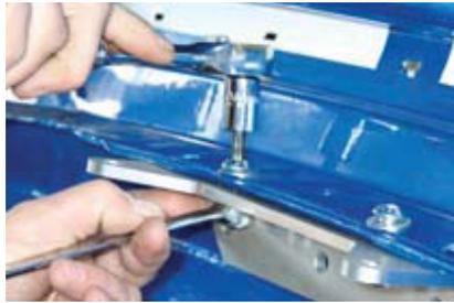
**2** The billet firewall bracket is next, with screws kept loose until installation is complete. Keeping them loose allows for adjustment when it's time to drill the firewall.
