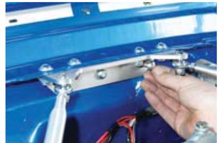
**15** Installation of the firewall brace is performed by feel with one person inside underdash and someone on the engine compartment side to run bolts. The reinforcement plate offers firewall rigidity and solid structural integrity.
