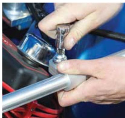
**13** Truss braces are next, which do not get spacers at the shock towers. The Heim joint is flush with the shock tower.
