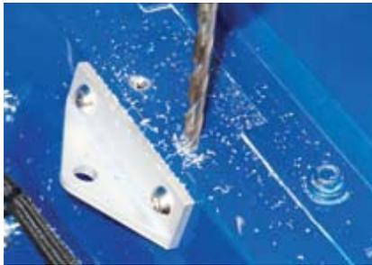
**10** Using the underside support bracket as a guide (pilot holes drilled first from underneath),  $\frac{3}{8}$ -inch bolt holes are drilled next from the top.
