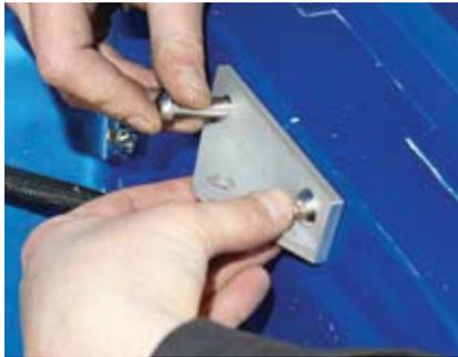
**9** Bolts are installed next along with the support bracket underneath.
