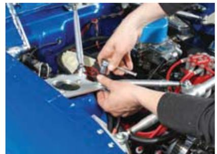
**16** The truss braces can be tightened at this time. Note the correct location of the shock tower brace spacer. The spacer goes between the shock tower Heim joint and bracket, not between the truss brace and bracket. This is an easy mistake to make.
