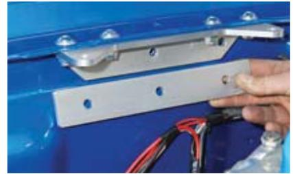
**14** The firewall brace is set up like this, with the reinforcement plate located behind the firewall.
