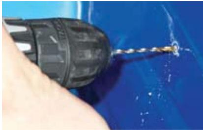
**8** Drill a pilot hole first as a guide, then drill  $\frac{3}{8}$ -inch holes.
