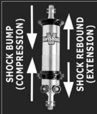
and inhibit weight transfer to the rear tires. By slowly adjusting the bump rate in on a set of double adjustable front shocks, you can adjust the rate that the front suspension settles after launch to prevent unloading weight transfer on the rear tires too quickly.
