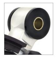
Rather than use the same mounting eye for urethane bushings and spherical bearings, VariShock's larger bushing eye accepts 350-percentmore material than conventional designs. The big bushing handles heavier loads and maintains the preload necessary to eliminate deflection and premature wear. This total redesign also required the creation of special molds, into which premium-quality urethane is poured.
