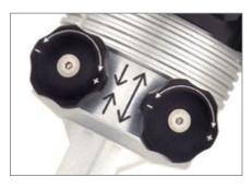
Machined arrows leave no doubt about which adjuster determines how firmly a VariShock comes together (bump) or pulls apart (rebound). Each knob offers 16 "full" settings — for a total of 256 valving combinations! Although competitors have added super-fine "half clicks" between stops to increase their advertised total, VariShock claims the widest adjustment range between "full soft" and "full hard."
