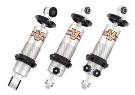
Billet-aluminum, clear-anodized coil-overs are offered in either (R-L) double-adjustable QuickSet 2; single-adjustable QuickSet 1; or nonadjustable SensiSet models. Eight different lengths allow shock travel from 2-3/4 to 9-3/4 inches. Note the revolutionary lower spring seat, which accepts a standard Allen wrench and utilizes a ball-locking mechanism. One-piece housing bases are machined with different mounts for spherical bearings or urethane bushings.
