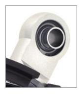
Clever engineering produced an exclusive bearing mount with longer, undercut eyes to maximize chassis clearance — without adding shock length or sacrificing travel. VariShock's Teflon-lined spherical bearing costs more, but prevents the sloppy fit of all-metal designs and short life of all-plastic races. It's also becoming popular in street applications.
