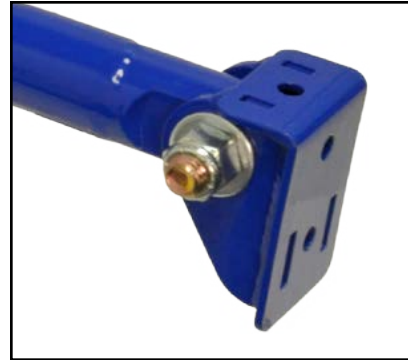
Weld-on frame brackets (2-3/4" tall) match Mustang and Nova rail height. Must be trimmed for shorter rail height of Falcons.
