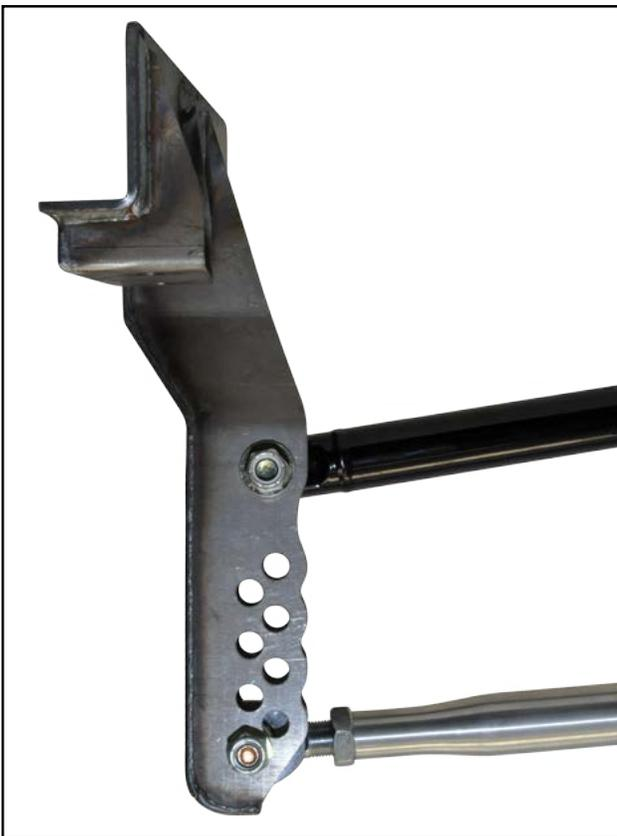
**Lower Positions (understeer)** - The lowest positions of adjustment tune toward a vehicle that understeers or pushes when cornering. This is considered to be a safe starting point.
