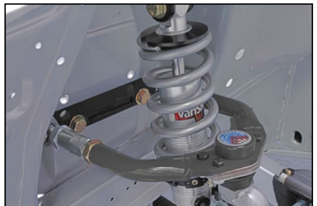
The greater incline created by the lower mounting position increases negative camber gain and reduces body roll.
