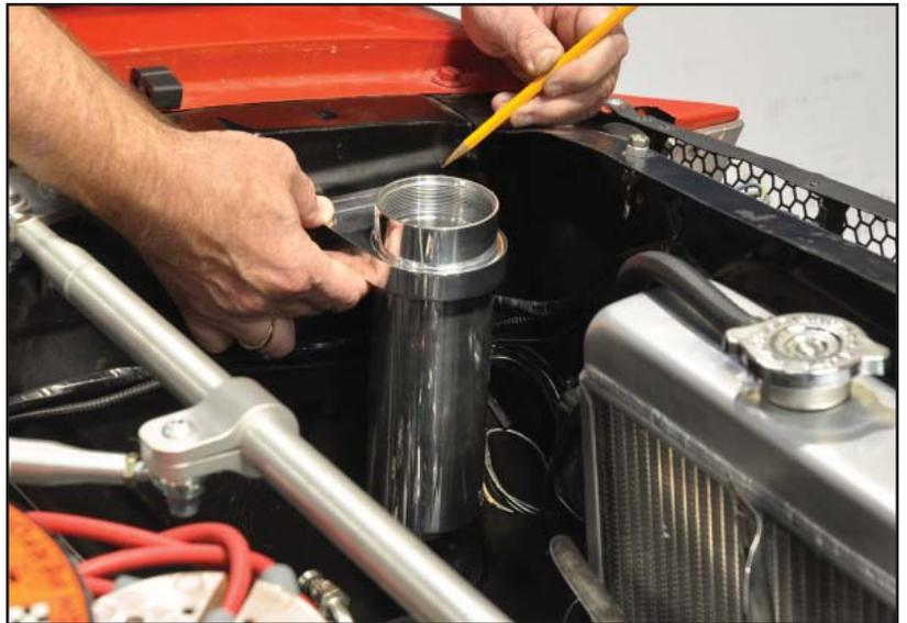
7. Use a ruler to measure the location of the two mounting holes in the adapter. The front hole is  $15/16$ " back from the front edge of the adapter, and the rear hole is  $2-15/16$ " back from the same front edge.
