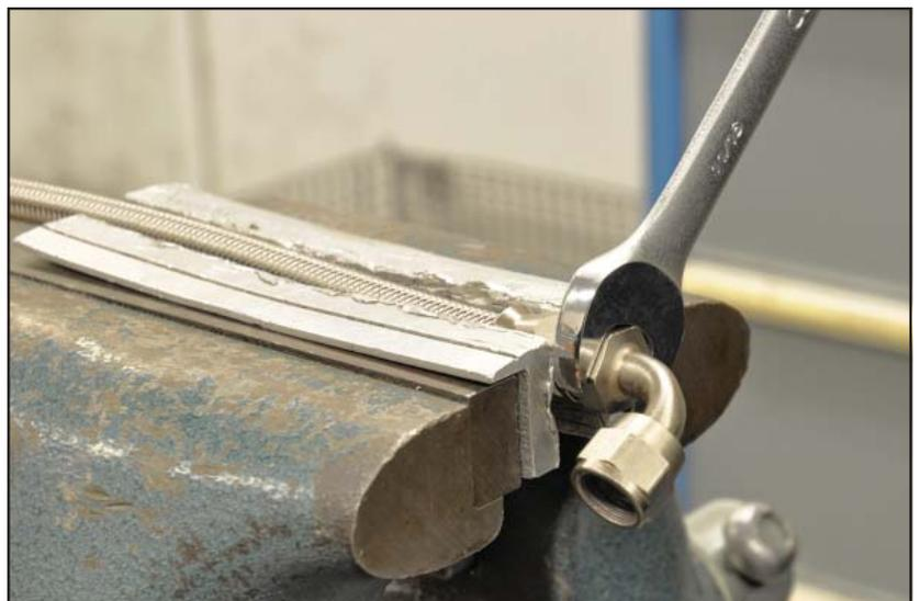
28. The fitting is assembled and we have lined up the tube of the fitting to a index mark. This is an important step because the fitting can not be rotated once they are tight.
