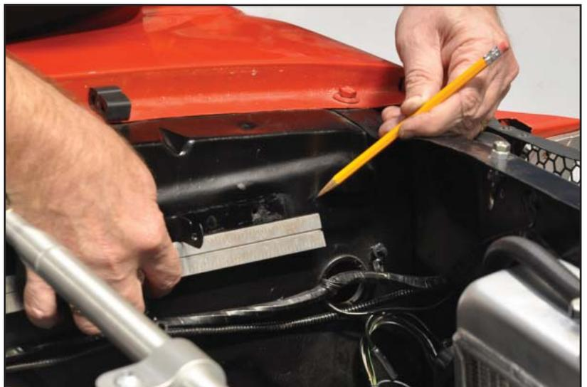
8. Check the area behind the hole locations prior to drilling. Make sure the locations are clear of wiring and are accessible for hardware installation.
