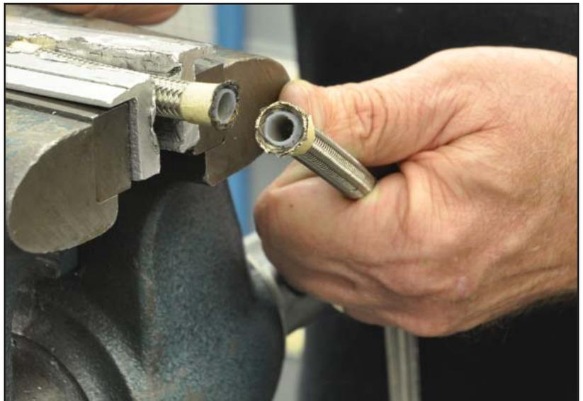
18. Disassemble the hose ends and slide the outer socket onto the hose with the threaded end of socket closest to the freshly cut end of the hose.
