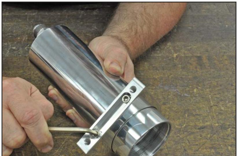
4. Next attach the 14 degree adapter, TCP PSR-01, to the billet clamp assembly with the socket-head cap screws provided.
