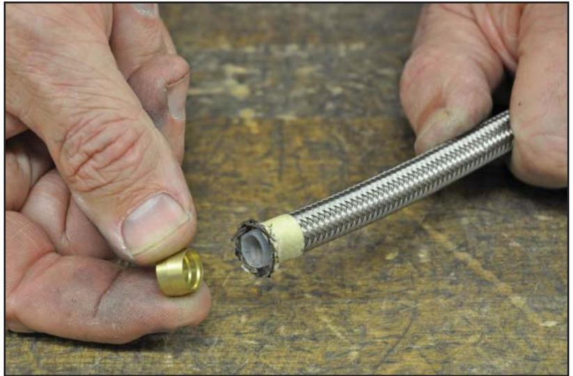
20. Apply pressure against the ferrule until the Teflon hose is seated against the inside lip of the ferrule.
