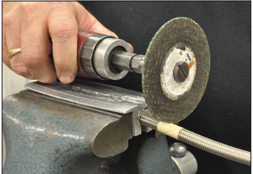
16. Clean inside of hoses thoroughly. Small metal and Teflon particles will damage the pump.
