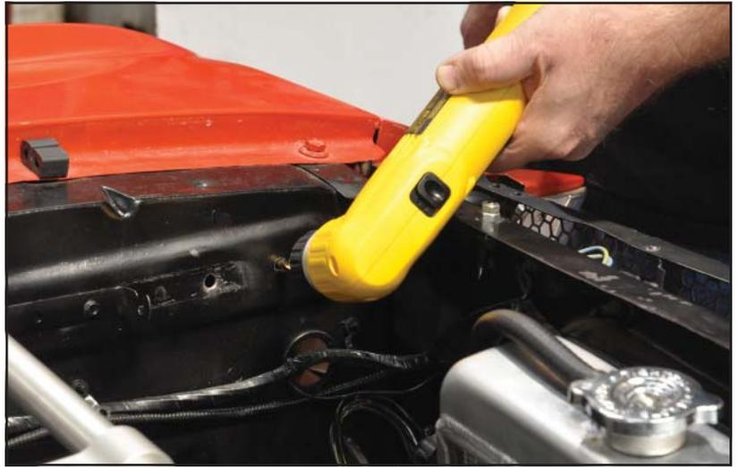
10. Secure the reservoir to the inner fender with the 5/16-18 x 1/2" button heads and flat washers supplied with the adapter.
