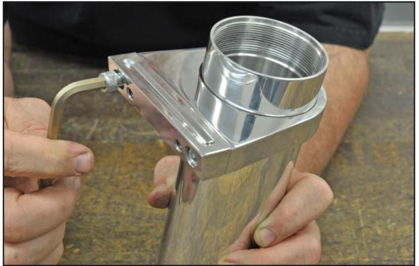
5. Position the reservoir on the inner fender, so when filled the fluid level is at least 2 inches above the top of the pump.
