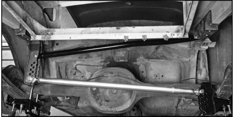
2. The passenger spring plate should already be installed. The anti-roll bar endlink will mount outboard of the leaf spring between the two tabs shown at far right of image.
