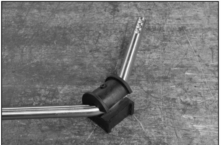
7. Place the billet housing over the bushing and screw in the grease zerk fitting.
