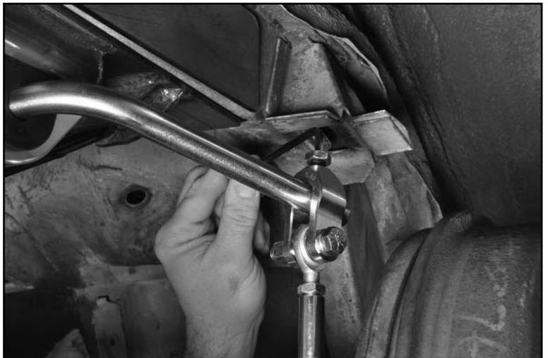
15. Attach the lower end of the endlink to the spring-plate clevis using 3/8" hex head bolt, aircraft washers and a locknut.
