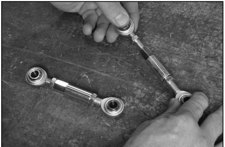
12. Attach the sliding-link clevis to each endlink assembly, using a 3/8" hex head bolt, two aircraft washers, and a locknut.
