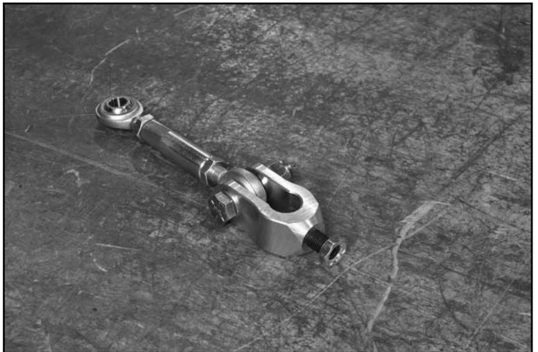
14. Attach the clevis onto the anti-roll-bar arms at the outermost detent. Tighten set screw, then jam nut. This position can be changed/adjusted later, but we begin at this position as the baseline.
