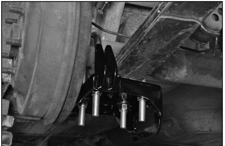
4. The bushings and billet housings are installed onto the bar before raising it into position.
