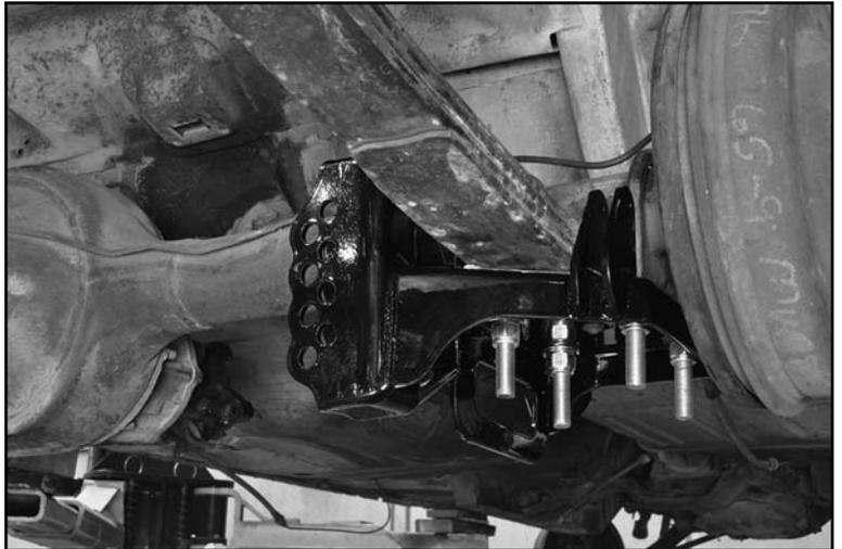
3. Install the TCP driver-side spring plate. Torque specification will depend upon U-bolt size. Continue with anti-roll bar assembly once all spring plate mounting hardware is tightened.
