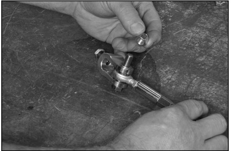
13. Start the set screw in the hole at the top of the clevis along with the jam nut.
