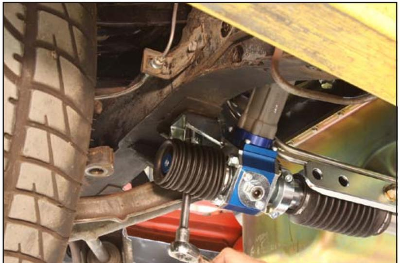
36. Loosely install each of the clamp collars (Item 2) onto their respective brackets so that the clamps seat against the rack tube to prevent rocking, but still allow rotation and sliding movement. A light lubricant can be used to more easily permit sliding of the brackets.
