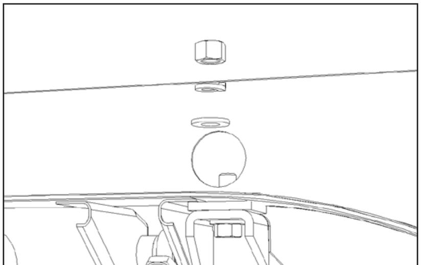
32. Raise rack and pinion assembly into position along brackets.
