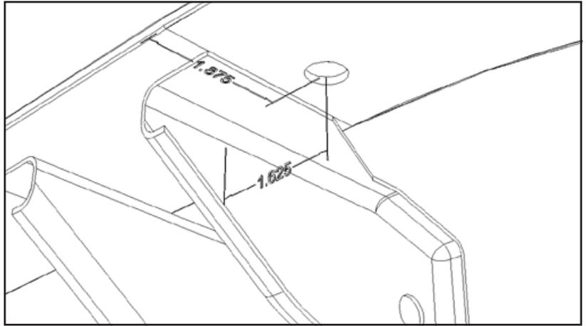
26. Using a 1-5/8" diameter hole saw, cut an access hole into the outside of the frame rail 1" directly above the 1/2" mounting hole.
