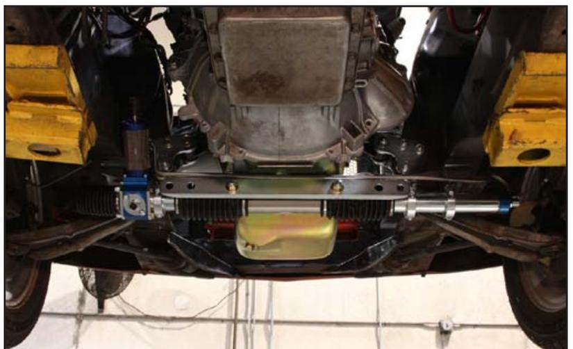
42. Verify that each of the three clamps are just tight enough to correctly align the bracket with the rack tube before lightly tightening the outer-bracket bolts into the frame rails.
