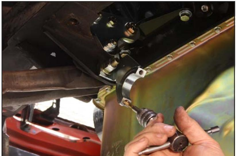
24. Drill a 1/8" pilot hole into the driver side frame rail, location of hole is shown in illustration.
