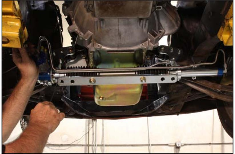
35. On driver-side frame rail, loosely bolt the rack and pinion's attached frame bracket to the hole drill in the frame rail, using the same hardware as the passenger side bracket.
