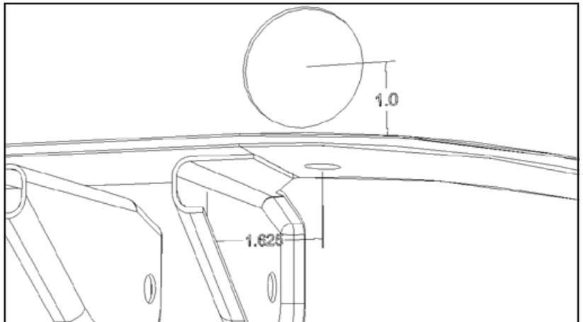
29. Loosely bolt frame rack bracket to mounting point on passenger side frame rail using 1/2-13 x2" hex bolt, lock washer and hex nut.
