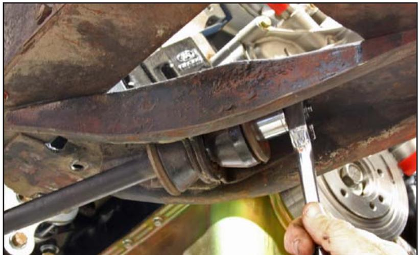
8. Remove the steel sleeve from the frame mount with a chisel. This may not on all vehicles.
