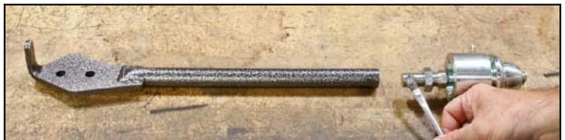
13. Remove button-head screw and backup nut from the pivot assembly.
