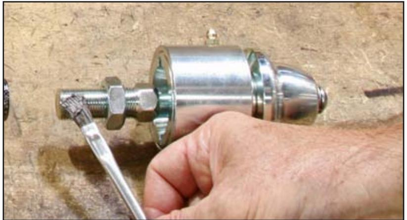
12. Screw pivot assembly into strut rod.
