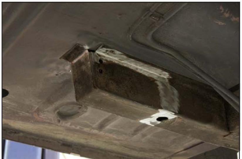
12. The rear frame rail must also be ground to bare metal along the marked line.
