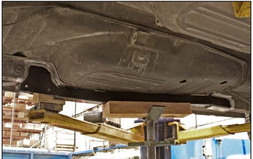
17. The front cup of the subframe connector must be seated tightly against the bottom and back edge of the factory frame rail.
