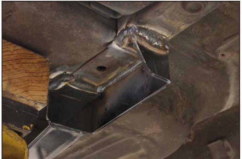
27. After the welds are completely cool, lightly scuff the bare areas with a scotch-brite pad and paint to protect from rust.
