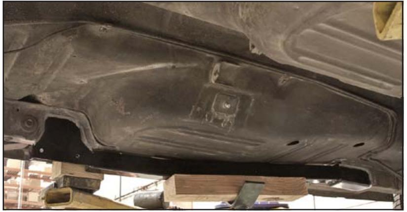
7. Using a marker or scribe, trace the outline of the frame connector plate along the inside of the frame rail.
