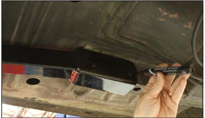
10. Use a disc sander or steel brush attachment and drill to remove any coating or grease that may be along the weld area of the front factory frame rails.
