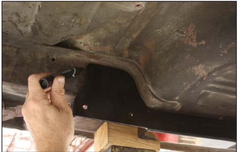
8. Trace the frame connector outline along the bottom of the frame rail
