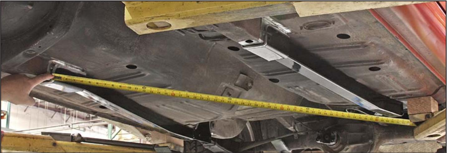
22. Once the connectors are square, tack weld the front and rear brackets of the loose connector.
