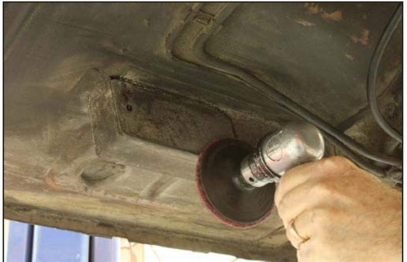
11. The marked area must be ground to bare metal to ensure a good clean weld.
