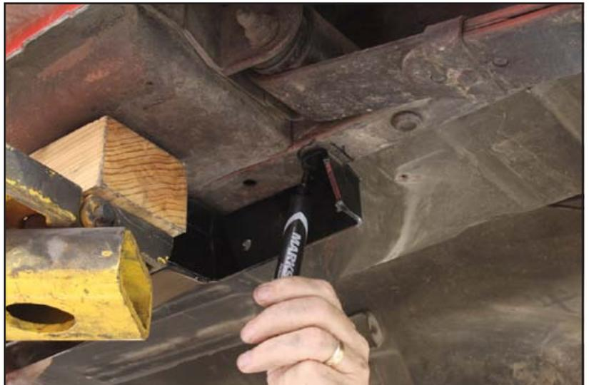
9. Trace the front frame connector cup outline onto the front frame rail.
