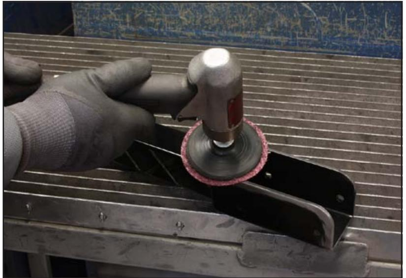
14. Bare metal must be exposed approximately 3/8" from all edges of the front cup.
