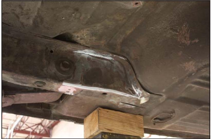
13. Remove the powder coating from the edges of the subframe connector where welds will be made.
