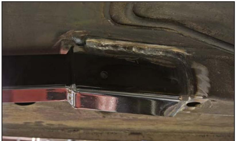
25. The rear bracket is welded along the top corner of the inside of the frame rail.
