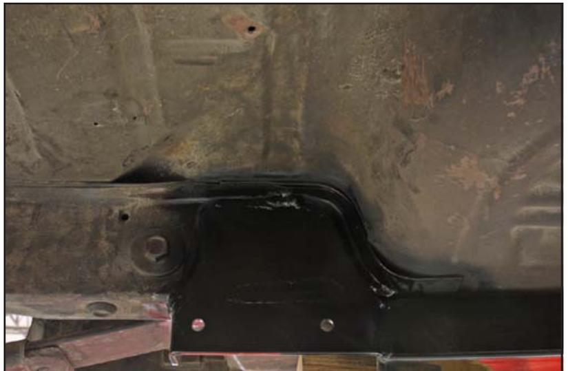
28. The subframe connector installation is complete. The connector support center section TCP SUBCS-01 can now be installed.
