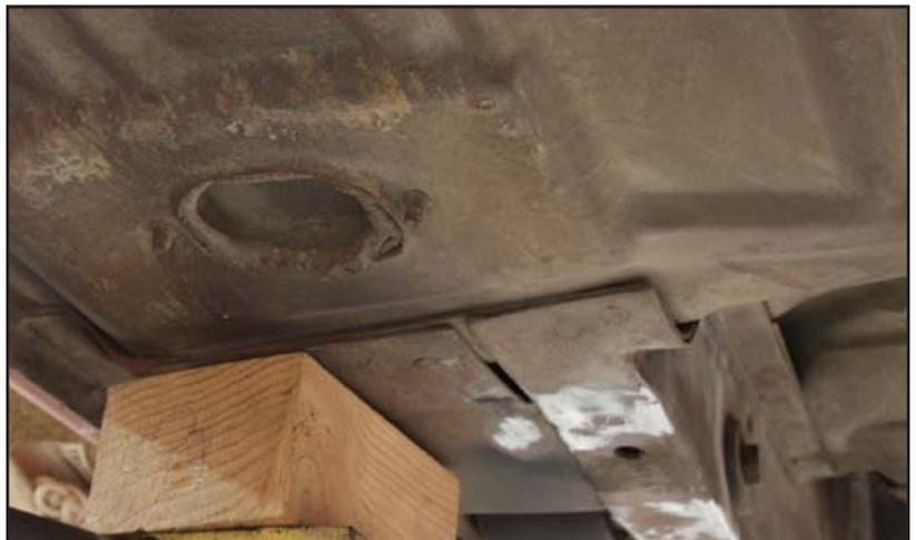
that lies against the frame rail. Grind a notch in the bracket wide enough to slip the front cup of the subframe connector into. The front cup should seat on the frame rail without interference from the bracket.
