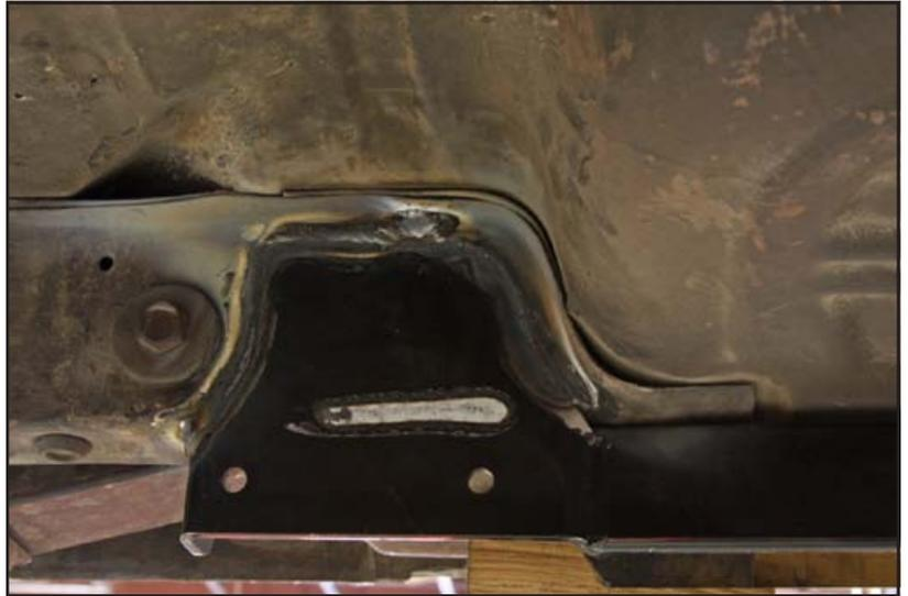
bottom of the frame rail and a bead is ran along the backside of the connector plate.
