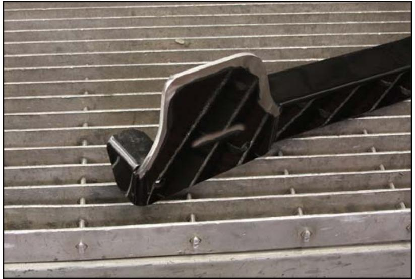
16. Raise the frame connector into position under the car and support it with a jack. The subframe connector is designed to seat directly against the floor pan for maximum ground clearance. It will take some pressure to fully seat the connector.
