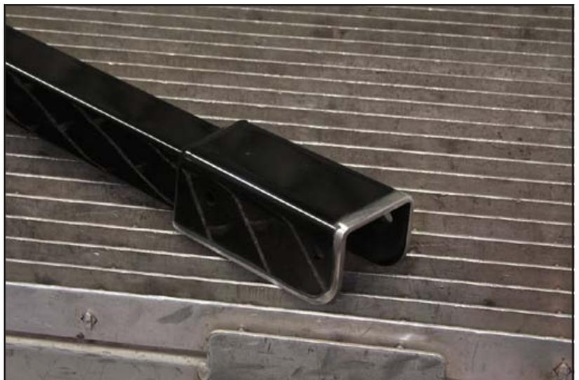
15. The rear connector bracket must be sanded around the large plate and along the smaller bent tabs that will sit underneath the frame rail.
