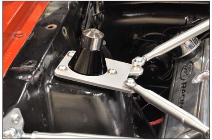
Bolt-On Coil-Over mounted BELOW - standard ride height
