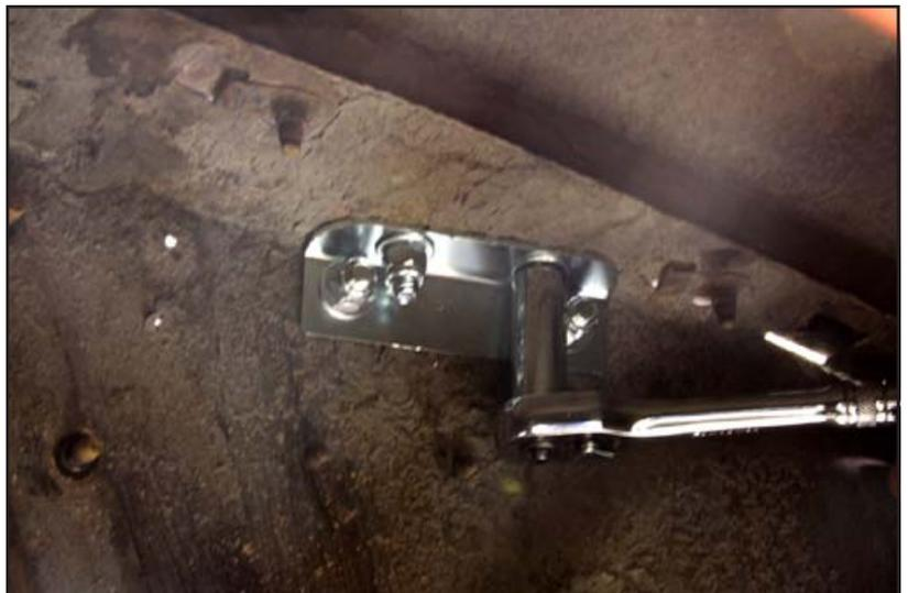
13. This is the completed fender bracket install on the passenger side.
