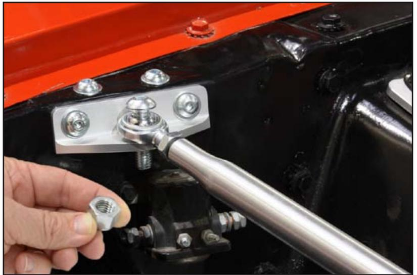
20. Tighten the fasteners to 40 lb-ft.
