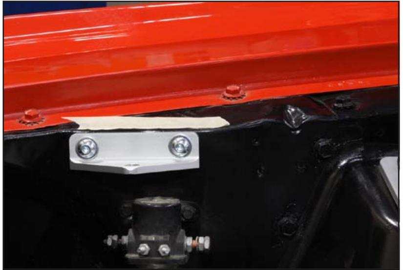
10. From underneath the fender, use the support bracket as a guide to drill 3/8" diameter holes through the inner fender.
