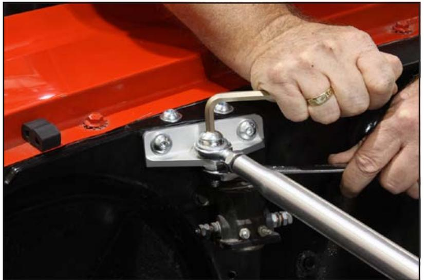
21. The length of the radius-rod assembly will have to be adjusted to line up with the second bracket. Hold the loose rod end to prevent it from rotating while adjusting. Thread engagement of each rod end must remain equal.
