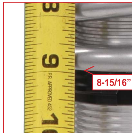
Measure the bottom end of the spring.
