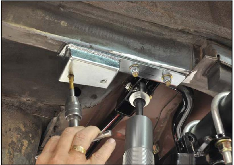
6. Raise the anti-roll bar with bushings and mounts into position against the vehicle. Detents in arms must be on top with arms extending toward front of vehicle.
