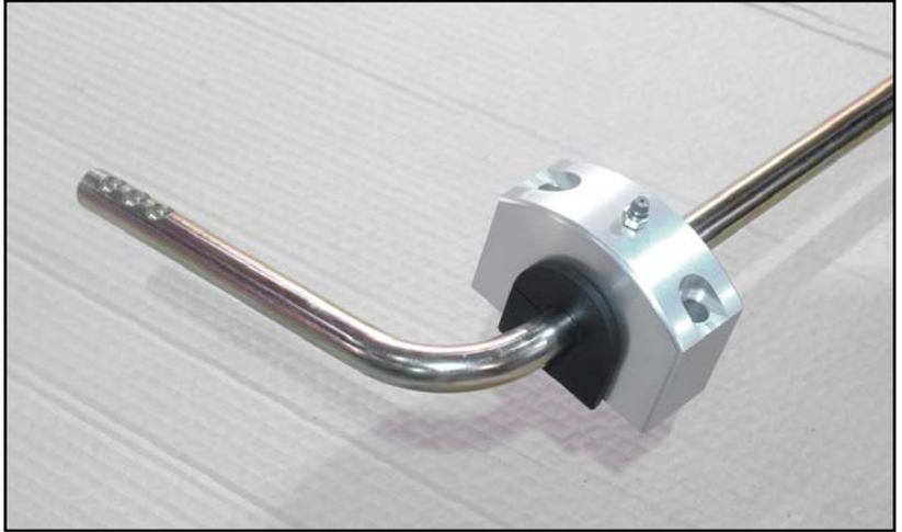
5. Use a 3/8-16 tap to chase the threads in the anti-roll bar frame mounts.
