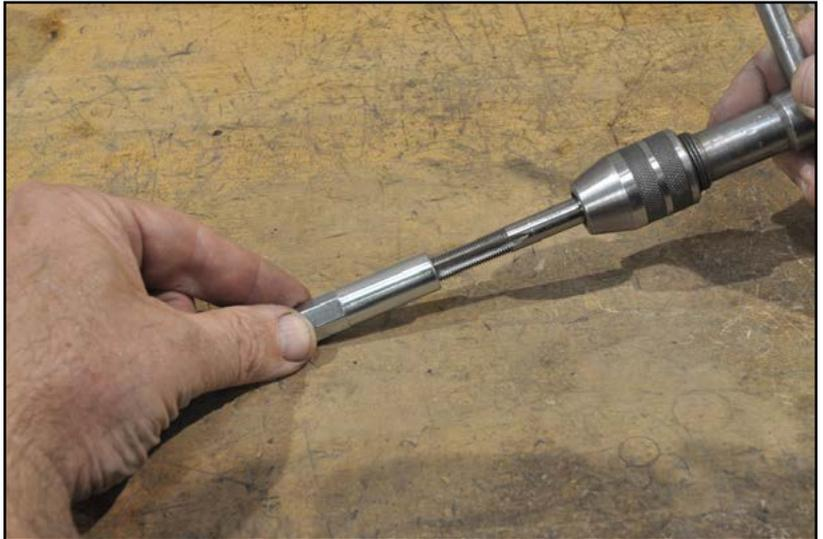
10. Thread the 3/8" jam nuts on to the male rod ends, leaving 5 to 7 threads showing between the jam nut and rod end body.
