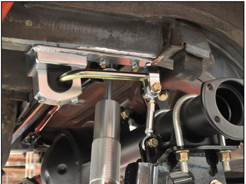
19. Rotate each rod end body so that it is centered within its clevis, then tighten jam nuts.
