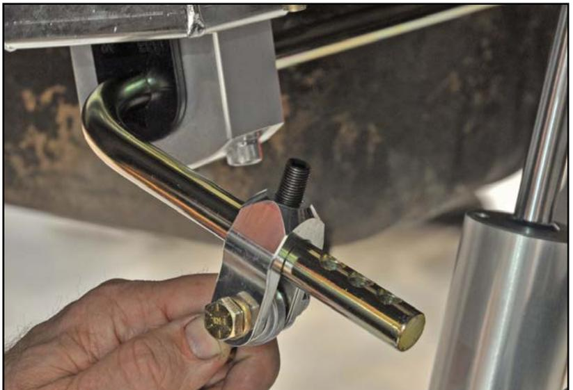
16. Bolt the opposite end of each adjuster endlink assembly to the tabs on the lower axle brackets, using 3/8-24 x 1-3/4" hex bolts, aircraft washers and locknuts.
