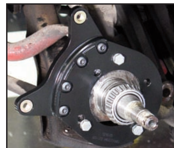
Photo 2 (Disc Spindle Mounting)
