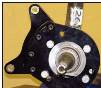
Photo 1 (Drum Spindle Mounting)
