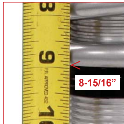
Measure the bottom end of the spring.
