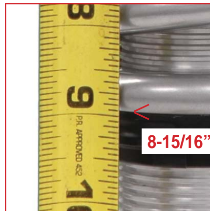
Measure the bottom end of the spring.
