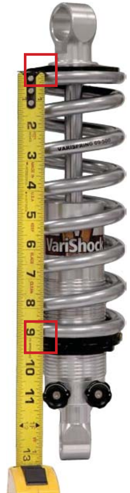
Measure the bottom end of the spring.
