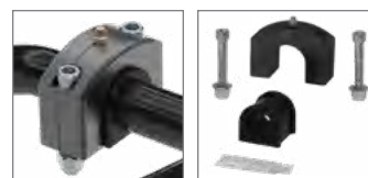
Crossmember-mounted bushing housing; poly or COM-8 lower end link
