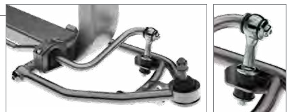
Crossmember-mounted bushing housing; poly-bushing lower end link
