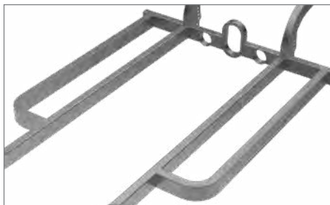
Straight-Rail Mid-Frame Parallel design works well for short or narrow chassis
