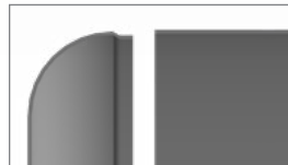
Offset tub-cap lip seats underneath edge of tub skin, creating an easy to align overlap joint with flush outer surface.
