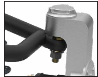
Upper Arm Pivot - Housed within the billet upright, the tension-adjustable pivot assembly can be tightened to compensate for wear.
