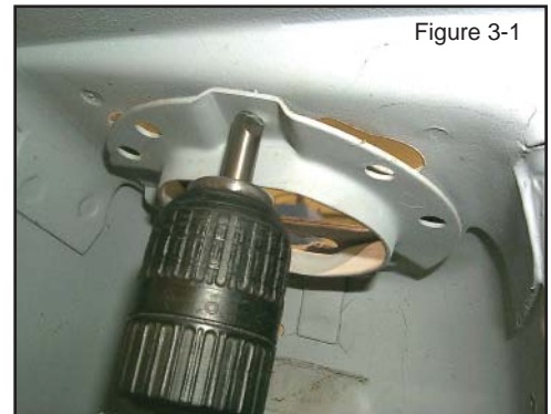
Figure 3-1 applies only to vehicles using carriage bolts to secure the factory upper shock mount.
