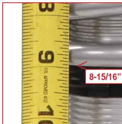
Measure the bottom end of the spring.
