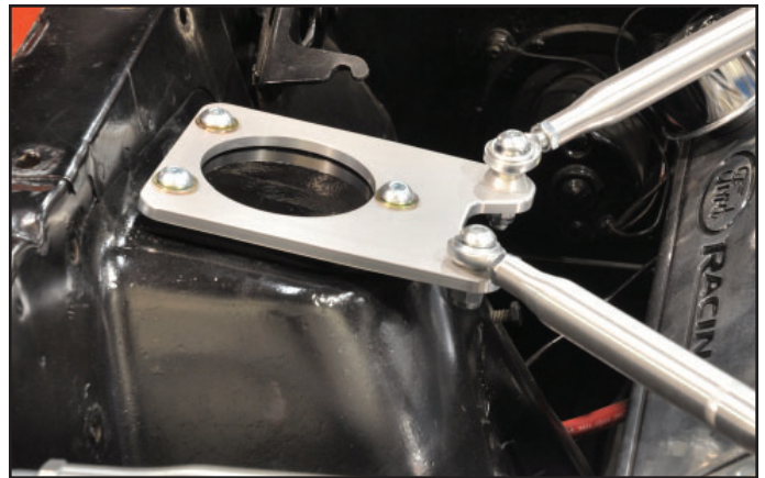
Full Coil-Over mounted BELOW - standard ride-height
