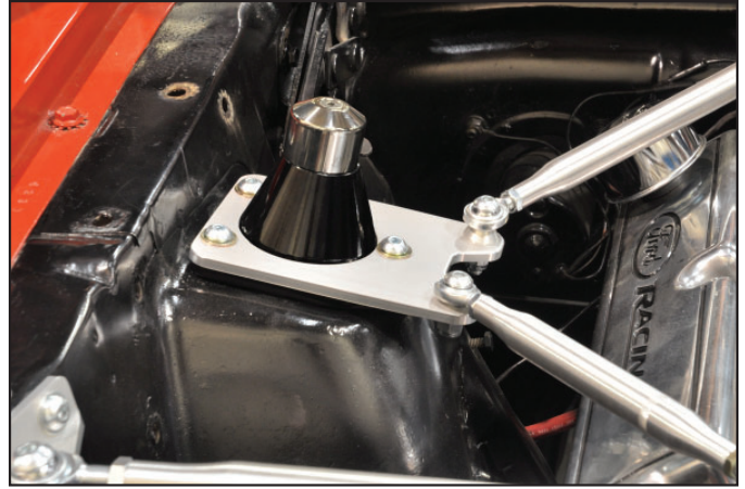
Bolt-On Coil-Over mounted BELOW - standard ride height
