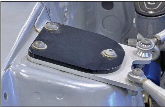
Full Coil-Over mounted ABOVE - lowered ride height
